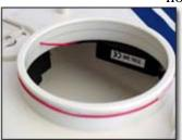
Photo #5: Wrap wire around the outside of the conning tower without crossing the wire over itself. It should lie flat in bottom of groove. If you have a 75 mhz radio, it will go around just once. A 27 mhz wire will go around more than once. Either tape or silicon glue
