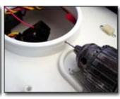
Photo # 2: Drill a 1/16" in the aft side of the "conning tower" right at the bottom of the groove.
