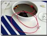
Photo # 1: Remove antenna from original mount, pull antenna wire below, seal up old deck antenna mount hole.
