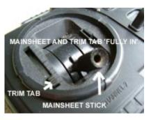
sailing position. The correct position is with the trim tab in the central position). The mainsheet attachment loop on the sheeting system should now be somewhere near the bow unless you have had a complete unwind of the sheeting system.
